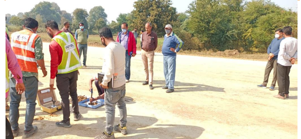
FDD checking on Embankment bed during site visit of AE
